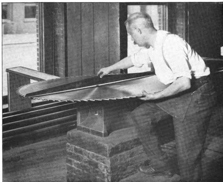
Fig. 71. Appearance of a saw having correct tension.
